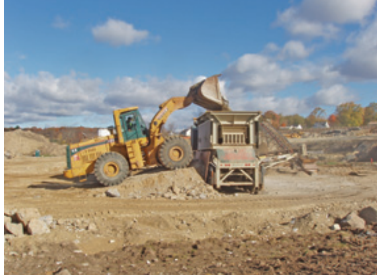
Nationwide Rock and Recycling Corp.'s Kawasaki loads rock into a Lippman 30 X 48 jaw crusher.
